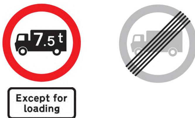
Images 3 and 4: Signs used at the start and end of a 7.5 tonne weight limit
